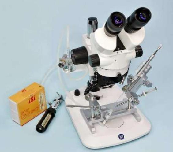
A white stereo microscope with two eyepieces, mounted on a base. To the left is a yellow box labeled 'ISI Bear Chargers' and a black screwdriver.  | <p><b>Strumento completo 1.02 StereoBlue Zoom</b><br/>Pronto all'uso</p> <p>con microscopio StereoBlue Zoom 7-45x, oculare HWF 10x/20 mm , illuminazione LED,<br/>siringa SCHLEY,<br/>pinze a pressione e anestesia.</p> |  |
